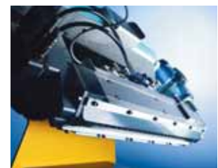
ProFlow® enclosed print head technology
