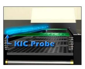
KIC 探测器: length and TC spacing is customized to each oven
