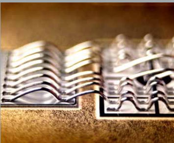
Defect detection on mul- tiple wire connections and multiple loops
